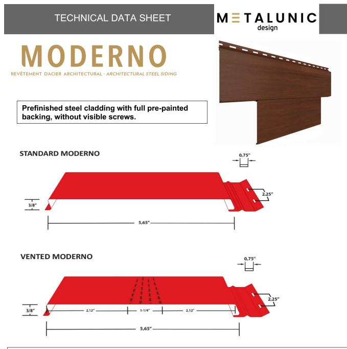
Provides ~33 sq. in. (0.021 m2) of ventilation opening per panel ; 3.375 sq. in. / linear foot (0.218 m2 / linear m)
